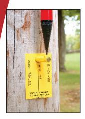
The BENCHTIE will save you time and money by allowing all benchmarks and ties to be plotted on work sheets for easy reference. The BENCHTIE is designed to be used with the information tag. Once the BENCHTIE is set and located, information can be recorded on the tag with a permanent marker. This will enable the surveyor to leave a benchmark that is easily identified and used by others.
