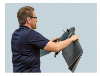
Upload your flight plan wirelessly to your drone. After a simple hand launch, your eBee X drone will then fly, capture images and land by itself.
