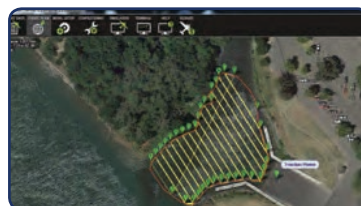
Preplanned survey using Mission Planner
