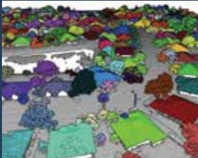
The Segmentation tool analyzes the characteristics of points in order to identify clusters and apply a Segment ID that can be visualized, searched, and selected.
