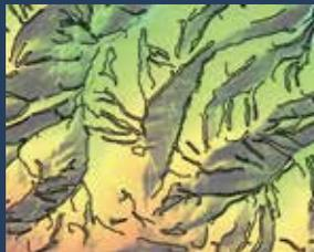
The new breakline extraction tool in Global Mapper Pro finds changes in elevation or slope and extracts these edges as 3D vector breaklines.
