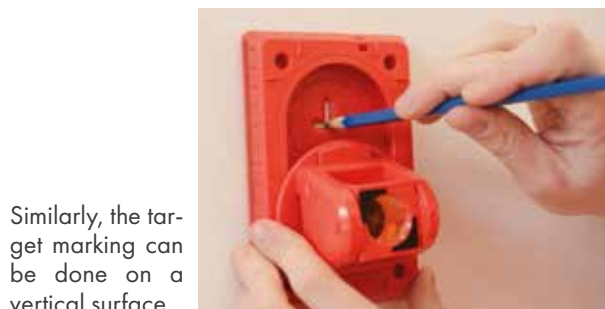
Slide the prism to one side and mark the target position with a pencil.
