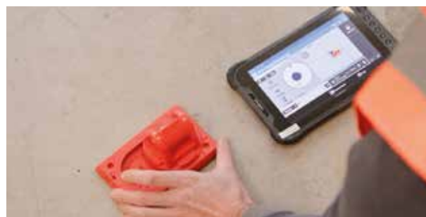
Move the stake out aid on the base plate until the target position is reached – visible on the green circle.
