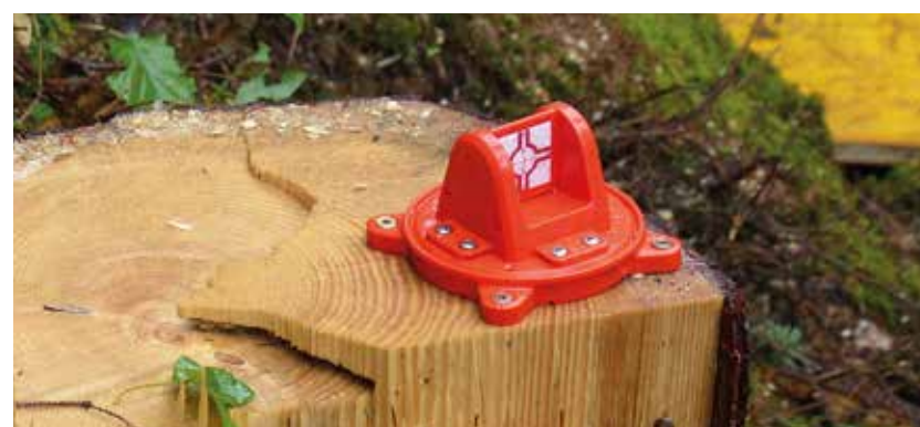
Example of the use of RS193M* as a fixed point on different surfaces and for the exact alignment of the drill carriage.
