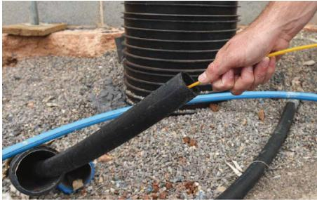
The FlexiTrace reel holds 164' (50m) or 262' (80m) of small diameter rod. The flexible rod can be energized by a transmitter and inserted into pipes as small as 0.5" (12mm).
