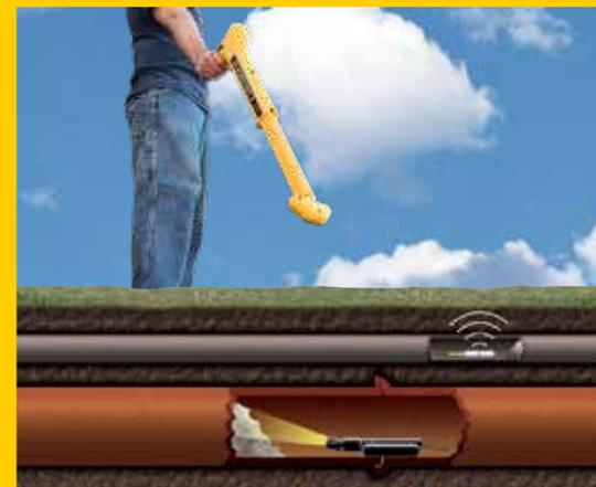
*"I don't use a sonde often, but things went perfectly! We taped the sonde to a jetter and tracked it as it was fed down the line (which went under a business that was built over a section of the pipeline after it was laid). Once I pinpointed the sonde with the XT receiver, we further pinpointed it with the Schonstedt magnetic locator they already owned."*
